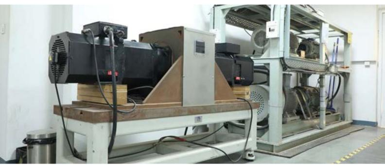
LTTS' Motor Dyne system conducts troubleshooting of power electronics
